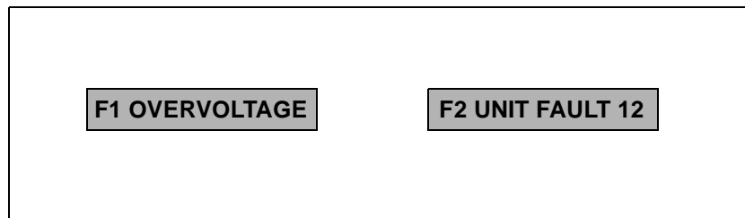
Figure 8-1 Examples of fault indications in the fault memory.
