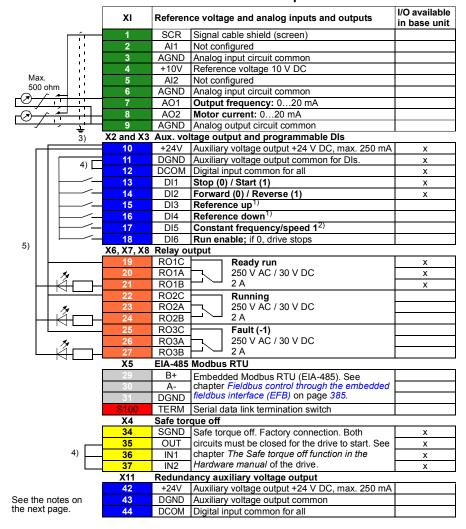
Tightening torque: 0.5 N·m (0.4 lbf·ft)
