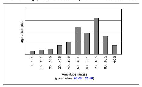
Amplitude logger 1 is fixed to monitor motor current, and cannot be reset. With amplitude logger 1, 100% corresponds to the maximum output current of the drive  $(I_{max})$ , which is listed in the *Hardware manual*. The measured current is logged continuously. The distribution of samples is shown by parameters 36.20...36.29.
