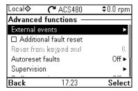
The Advanced functions submenu contains settings for advanced functions, such as triggering or resetting faults via I/O, signal supervision, using the drive with timed functions, or switching between several entire sets of settings.
