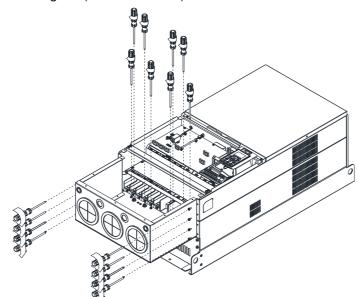
Fasten all the screws. Screw torque: 24~26kg-cm (20.8~22.6lb-in).
