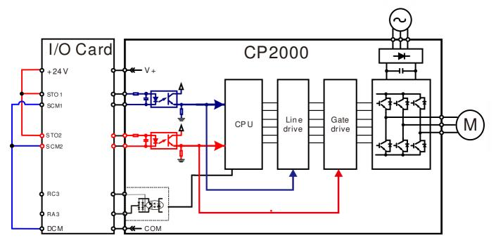
20-3-3 The control loop wiring diagram:
