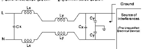
A filter is composed of a Differential Mode section (to eliminate noise below 150kHz) and a Common Mode section (to eliminate noise above 150kHz). For high-frequency noise, the inductor acts as a high impedance to form an open circuit and the capacitor acts as a low impedance to form a short circuit. Proper design and dimensioning of inductors and capacitors give a resonant circuit to absorb harmonic currents. Capacitor Cy is earthed to lead the harmonic currents to the ground.
