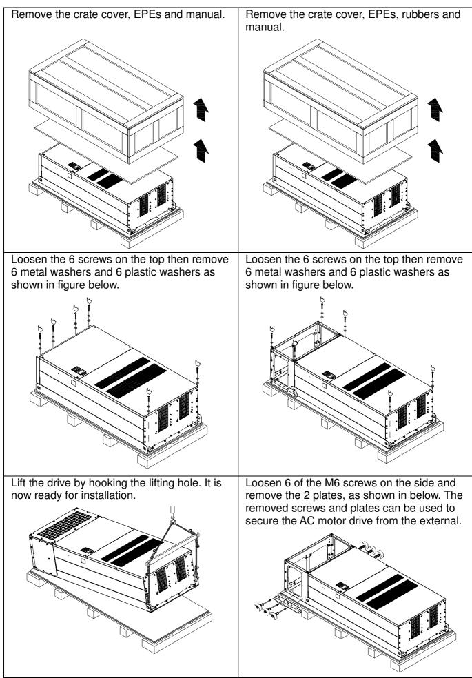
Secure the drive from the external. (Skip to the next step if it is not necessary in your case) Loosen 8 of M8 screws on the both sides and place the 2 plates that were removed from the last step. And then fix the plcates to AC motor drive by fasten 8 of the M8 screws. (As shown in below) Torque: 150~180kg-cm [130.20~156.24lb-in.] Lift the drive by hooking the lifting hole. It is now ready for installation.
