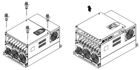
2. Fasten the 6 screws shown in the following figure and place the cover back to the original position. Screw torque: 24~26kg-cm (20.8~22.6lb-in).
