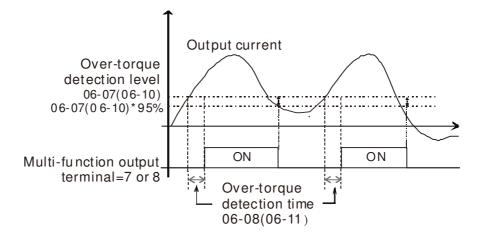
When Pr06-06 or Pr06-09 is set to 2 or 4, the motor drive will have the ot1/ot2 fault after Over Torque Detection. Then the motor drive stop running until it is manually reset.
