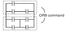
In the case of ANB and ORB operations, if a number of blocks are connected, they should be combined to form a block or network from the top down or from left to right.
