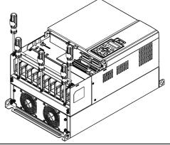
3. Install the conduit box by fasten the 5 screws shown in the following figure. Screw torque:24~26kg-cm (20.8~22.6lb-in)
