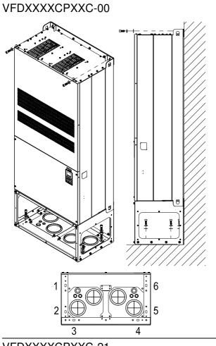
Secure the drive from internal. Screw: M12\*8 Torque: 340-420kg-cm [295.1-364.6lb-in.]
