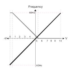
Pr.00-21=0 (Dgital keypad control and d run in FWD direction) Pr.03-05 Analog Positive Voltage Input Bias (AVI2) = 10% Pr.03-07~03-09 (Positive/Negative Bias Mode)
