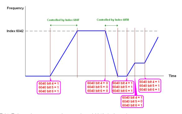
NOTE 01: To know the current rotation speed, read 6043. (unit: rpm) NOTE 02: To know if the rotation speed can reach the targeting value; read bit 10 of 6041. (0: Not reached; 1: Reached)
