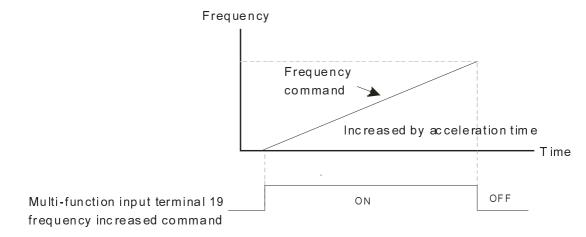
Pr.02-09 set to 1: use multi-function input terminal ON/OFF to increase/decrease the frequency command(F) according to the setting of Pr.02.10(0.001~1.000Hz/ms).
