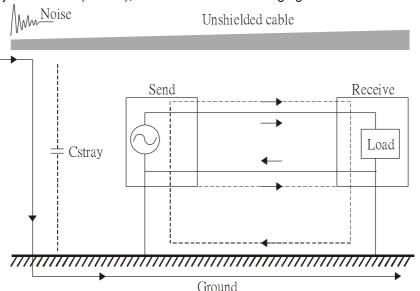
2. Common-mode noise in the power cable is transmitted through the stray capacitance and coupled into the adjacent signal cable, as shown in Figure 2. Several methods can be applied to reduce the effect of this common-mode noise; for example, shield the power cable and/or the signal cables, separate the power and signal cables, take the input and output side of the signal cable and twist them together to balance out the stray capacitance, let power cables and signal cables cross at 90°, etc.
