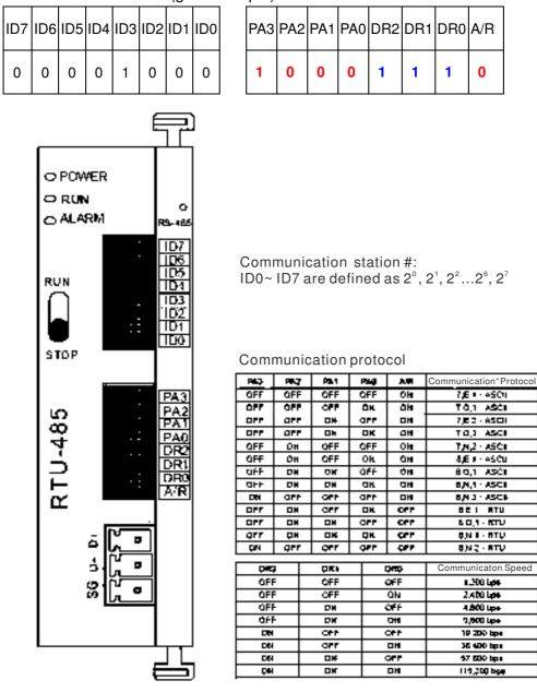
Step 2: Install control equipment. We sequentially connect a DVP16-SP (8 IN 8 OUT), DVP-04AD (4 channels AD), DVP02DA (2 channels DA), and DVP-08ST (8 switches) to the RTU485. The following corresponding locations can be obtained from the RTU485's configuration definitions:
