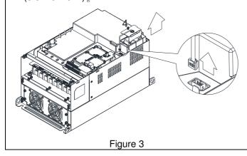
(Figure 2) Loosen screw 3, press the tab on the right and the left to remove the cover. Screw 3 <sup>[7</sup> Torque : 6~8kgf-cm (5.2~6.9lb-in) <sup>[</sup>
