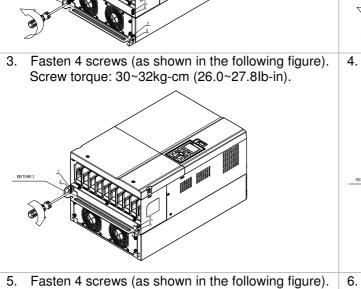
Fasten 4 screws (as shown in the following figure Screw torque: 24~26kg-cm (20.8~22.6lb-in).
