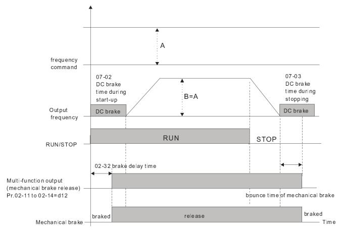
If this parameter is applied without DC brake, it will be invalid. Refer to the following operation timing.
