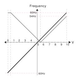
Pr.00-21=0 (Digital keypad control and d run in FWD direction) Pr.03-05 Analog Positive Voltage Input Bias (AVI2) = 10%
