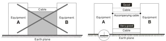
In order to avoid "Common Mode Noise", please use parallel wires or twisted pair wiring. Follow this rule and also avoid long wires, it is suggested to place the two wires as close to each other as possible.
