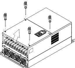
2. Install the conduit box by fastens the 4 screws, as shown in the following figure. Screw torque: 24~26kg-cm (20.8~22.6lb-in).
