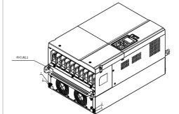
Place 4 screws (M10) through Fixture 1&2 and the plate then fasten the screws. (as shown in the following figure) Frame D0/D M10\*4 Screw torque: 200~240kg-cm (173.6~208.3lb-in). Frame E M12\*4
