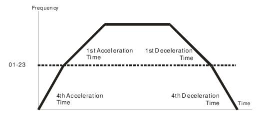
1st/4th Acceleration/Deceleration Frequency Switching
