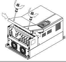
2. Remove the 5 screws shown in the following figure. Screw torque:24~26kg-cm (20.8~22.6lb-in)
