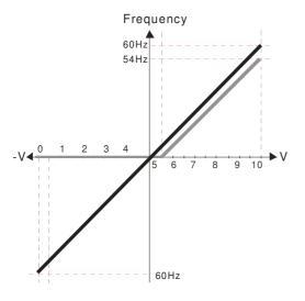
Pr.00-21=0 (Digital keypad control and run in FWD direction ) Pr.03-05 Analog Positive Voltage Input Bias (AVI2) = 10% Pr.03-07~03-09 (Positive/Negative Bias Mode)
