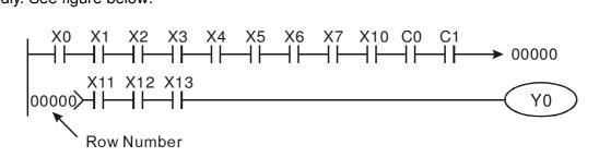
The ladder diagram programming method involves scanning from the upper left corner to the lower right corner. The coils and applications command computing box are handled in the output, and the ladder diagram is placed on the farthest right. Taking the figure below as an example, we can gradually analyze the procedural sequence of the ladder diagram. The number in the upper right corner gives the sequential order.
