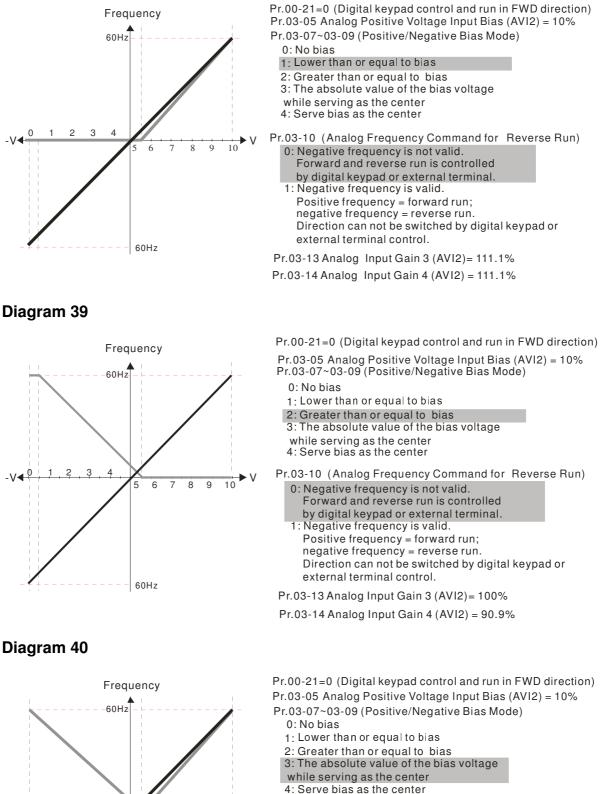
Pr.03-10 (Analog Frequency Command for Reverse Run) 0: Negative frequency is not valid.
