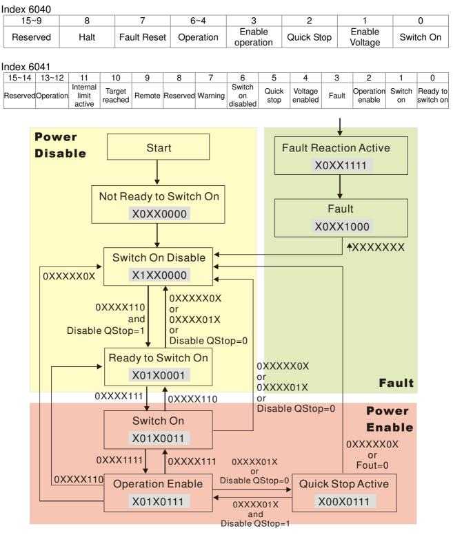
Set command 6040 =0xE, then set another command 6040 =0xF. Then the motor drive can be switched to Operation Enable. The Index 605A decides the dashed line of Operation Enable when the control mode changes from Quick Stop Active. (When the setting value is  $1 \sim 3$ , this dashed line is active. But when the setting value of 605A is not  $1 \sim 3$ , once he motor derive is switched to Quick Stop Active, it will not be able to switch back to Operation Enable.)
