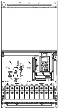
Main circuit terminals: R/L1, S/L2, T/L3, U/T1, V/T2, W/T3, +1/DC+, -/DC-
