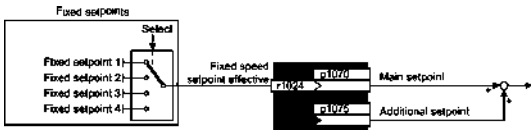
Figure 9-12 Fixed speeds as setpoint source
