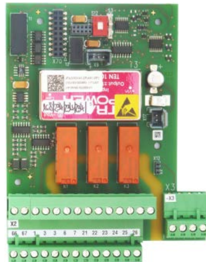
Peripheral board DI/DO
