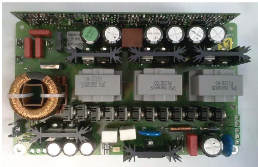
Figure 3-12 PC board of the pre-switch mode power supply (pre SMPS 300W)
