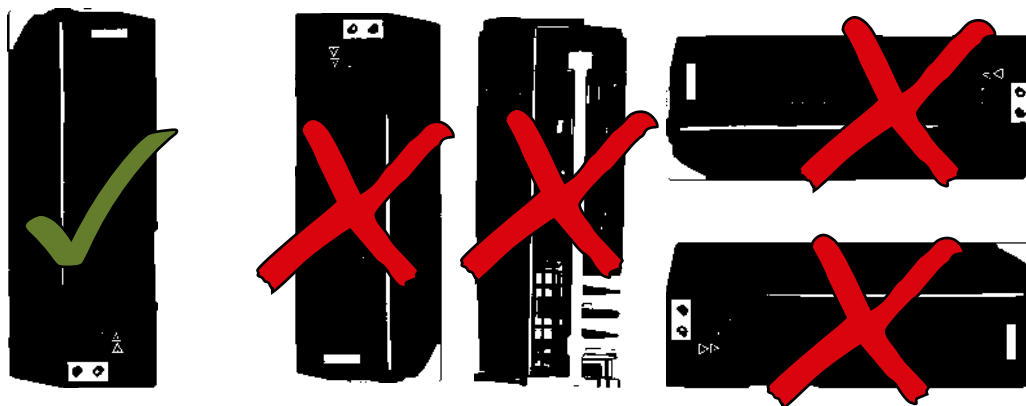
Figure 5-2 Mounting position of the converter
